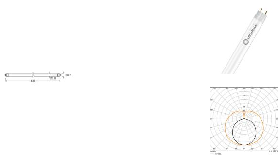
**Scheda tecnica Ledvance Tubo LED T8 EM Superior Conventional (EM), Mains (AC) Standard Output 5.1W 900lm - 840 Bianco Freddo | 44cm - Sostitutiva 15W**
